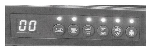
If machine has timed out, cycle machine off/on (position "1") again and allow to auto fill. If machine is still timing out, shut machine down and re-check the inlet water line / filtration system and confirm water flow to machine.
