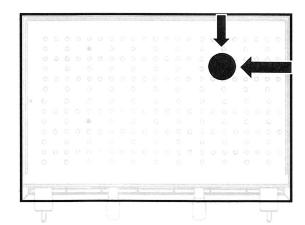
2.5" hole in counter recommended for passage of electrical cord & water/drain lines.
