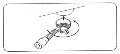
When the coffee grounds have to be emptied out, knock the filters against a wooden surface and not a metal one as this could damage the edge of the filter and jeopardize its tightness.
