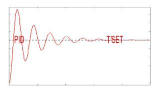
The three constants and the proportional range have to be adapted to the espresso machine, depending from the heating element power, the boiler dimensions, the fluidic and its dispersion. This regulation usually requires a bit of time in order to get the best possible result.
