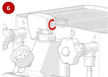
Screw the locking screw by using an allen key 2mm size.
