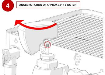
Rotate the paddle clockwise of 1 or more notches. (By moving the paddle of 1 notch, the water flow rate will increase approx. 1ml/sec.)
