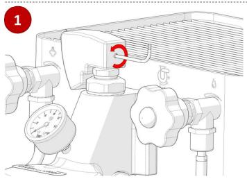
With the paddle completely to the left position, loosen the locking screw by using an allen key 2mm size.
