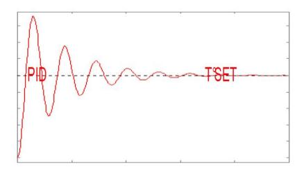
The three constants and the proportional range have to be adapted to the espresso machine, depending from the heating element power, the boiler dimensions, the fluidic and its dispersion. This regulation usually requires a bit of time in order to get the best possible result.
