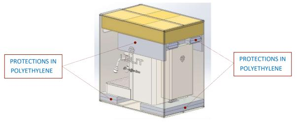
**3-** 8 corner angles in polyethylene have been inserted to space out the inner box from the overpack.
