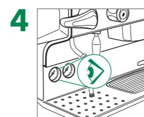
When the pressure is reached, wait for 10 min, in which there should be no increase of boiler pressure
