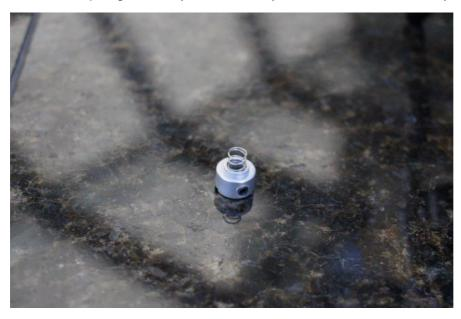
We have found forceps to be the absolute best tool, using other tools makes this process a lot more difficult. Use the forceps to compress the spring against the cylinder.
