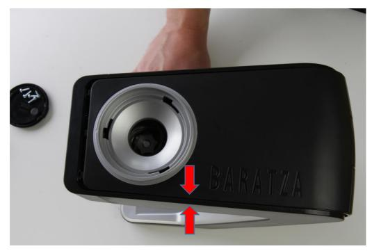
3. Work the case on such that it is flush with the sides and ready to slide forward to finish installation
