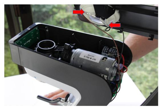
1. Slide the spade clips back onto the interlock switch.
