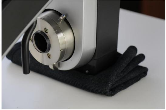
2. Remove the rear rubber foot (use pliers if needed)
