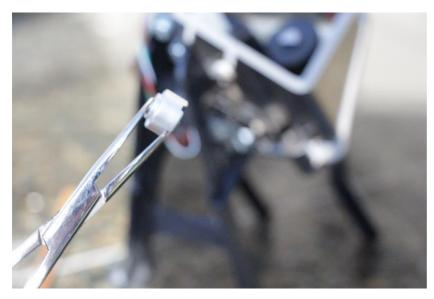
Here you can see the non-spring side of the cylinder and how nicely the forceps fit into the groove
