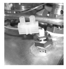
15. **Note:** once the water reaches the top of the boiler, some water will leak from the antivacuum valve (figure 1 below). You can address this issue by wrapping a twist tie around the nipple of the anti-vacuum valve (figure 2 below) in a way that the nipple will stick up mimicking the closed position of the anti-vacuum valve.
