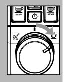
Turn the selector switch clockwise to set it to the "p" position. The machine rinse cycle starts.
