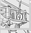
5 Wash the brew group with lukewarm water and carefully wash the upper filter. Before placing the Brew Group in its housing, make sure there is no water left in the brewing chamber.
