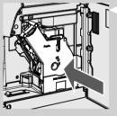
10 After rinsing the Brew Group, insert it again in its seat until it locks into place WITHOUT pressing the "PUSH" button.
