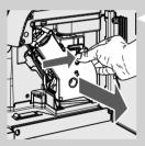
4 Remove the brew group: Pull it by the handle and press the «PUSH» button. The brew group must be washed only with lukewarm water with no detergent.
