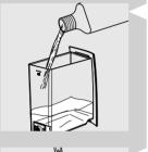
4 Pour the entire content of Saeco concentrated descaling solution into the appliance water tank.
