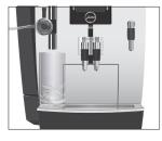
Coffee preparation starts. The preset amount of water flows into the glass. Preparation stops automatically. 'Please select product:' appears on the display.
