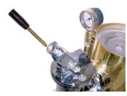
Screw pump lever clockwise into pump and hand tighten.
