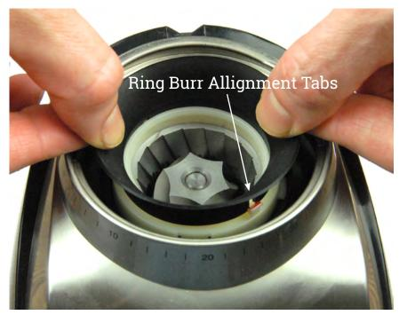
Ensure that the black adjustment ring is rotated counterclockwise as far as it will go. Replace the burr by lining up the
