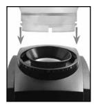
To replace the bean hopper, line up the two tabs on the base of the hopper (with the small tab on the right side) with their respective slots in the top of the grinder housing and insert the hopper into the grinder. Once the hopper is in place rotate it clockwise to your desired grind setting.
