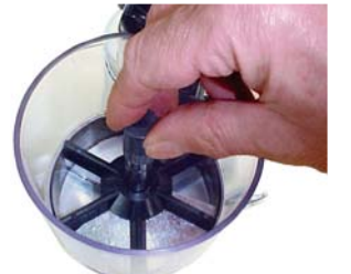
Adjusting the dose of coffee dispensed with each pull of the dosing lever
